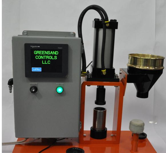
Optional Unit 2: GSC-PME-2001, Compactability Squeeze Pressure Calibration Kit- Contains load cell, load cell display and load cell holding fixture. This unit is used to read compression force in pounds at rod end of PME-ACTS.
